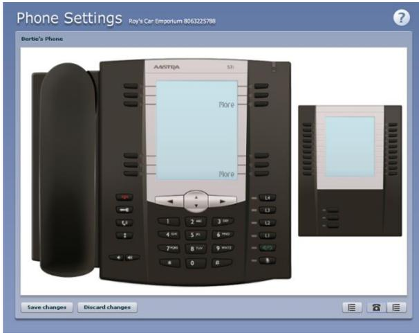
**FIGURE 64 PHONE CONFIGURATOR – PHONE AND SIDECAR VIEW**
